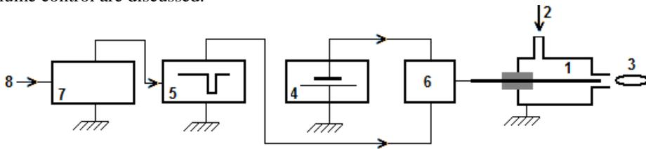
Fig.1: Experimental setup. 1-plasma source; 2-gas flow; 3-plasma plume; 4-dc voltage source; 5-high voltage pulses source; 6-voltage summing circuit; 7-driver circuit, 8-computer.
