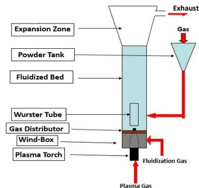
Fig1. The schematic of reactor
