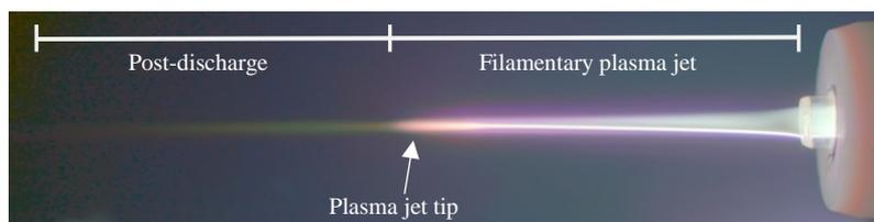
Figure 1. Image of the plasma jet with the filamentary component and the post-discharge
