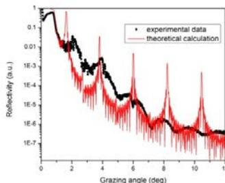
Figure 1. XRR spectra of a  $(W_{2nm}/Si_{2nm})_{18}$  stack: experimental data (black line) and theoretical calculation with no interlayer formation at the interfaces (red line)
