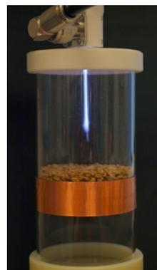
**Figure 1.** Image of the plasma jet and treatment chamber during operation
