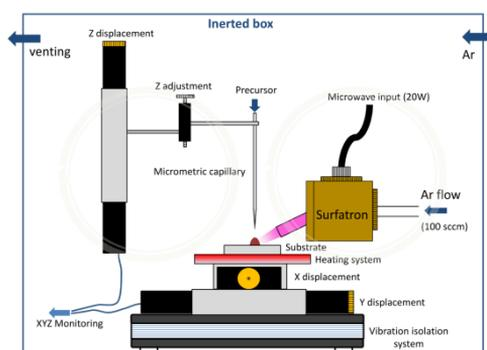
Schematic representation of the experimental device
