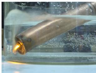
Figure 1. Image of plasma jet source sub-merged into liquid
