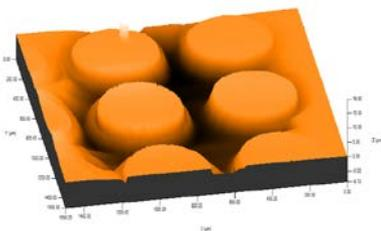
Figure 1. 3D image of pattern silicon surface etched in a mixture of Ar and SF<sub>6</sub> plasma for 10 minutes.
