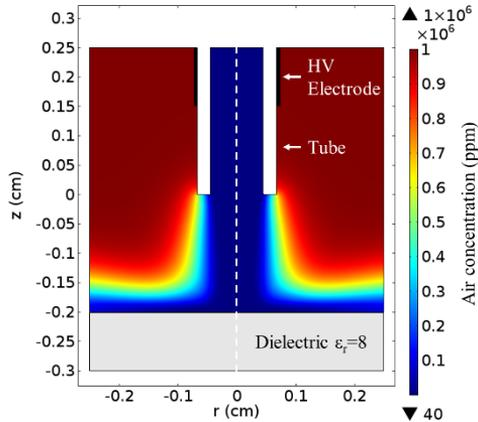
Figure 1: Simulation domain of the capillary plasma jet device and the air concentration (ppm) in the domain.
