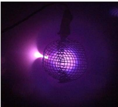
Fig. 1: Complex space-charge configuration inside and around a spherical grid cathode with hole
