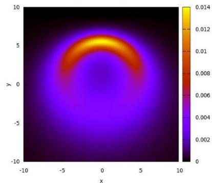
Figure 1. 3D profile of a film deposited on a substrate positioned at  $20^\circ$  in respect to the target (5 cm diameter) and 3 cm apart from it.
